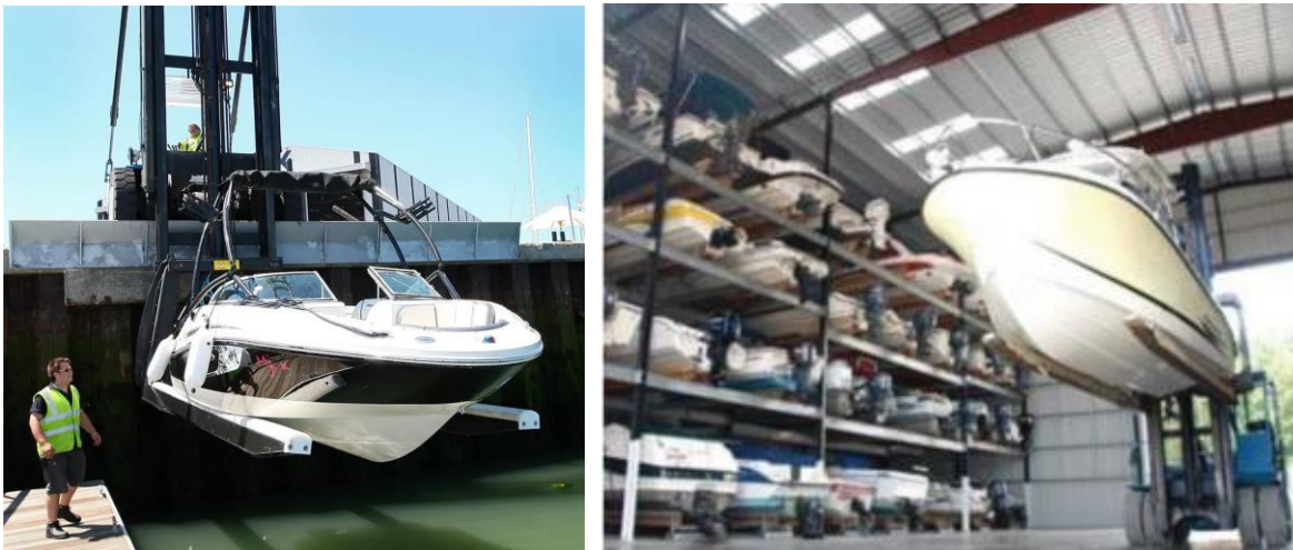
Figura 5.2: carrelli elevatori per Dry Stack Storage (negative fork lift)
