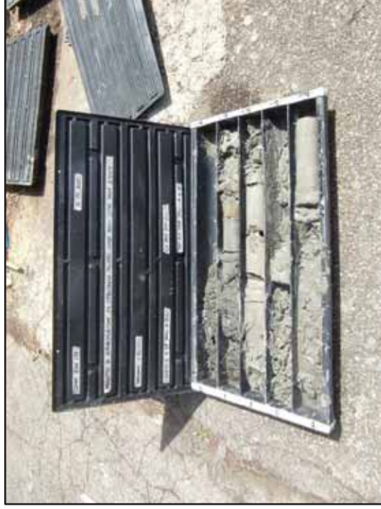
Foto n.20: SDH-01 – Cassetta 5 da 20,0 a 25,0 m
